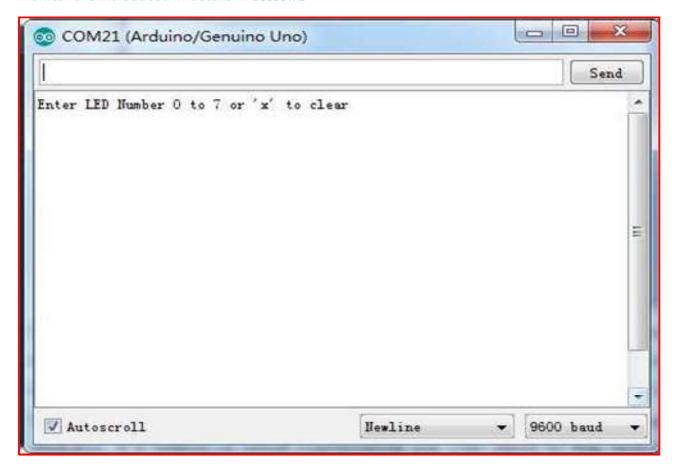
This window is called the Serial Monitor and it is part of the Arduino IDE software. Its job is to allow you to both send messages from your computer to an UNO board (over USB) and also to receive messages from the UNO.
