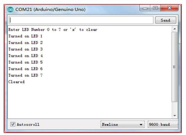
Type x again and press 'Send' to turn off all LEDs.
